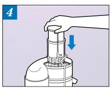
With the motor running, place food down the Feed Chute. Using the Food Pusher, gently guide food down the Feed Chute. To extract the maximum amount of juice, always push the Food Pusher down slowly. Do not force food down the Feed Chute. If food is stuck, turn OFF juicer and unplug. Remove food and cut food into smaller pieces.
